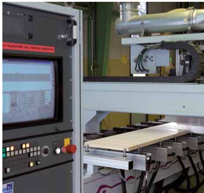
A computer-aided precision mill exactly transfers your draft to the wooden door panels.
